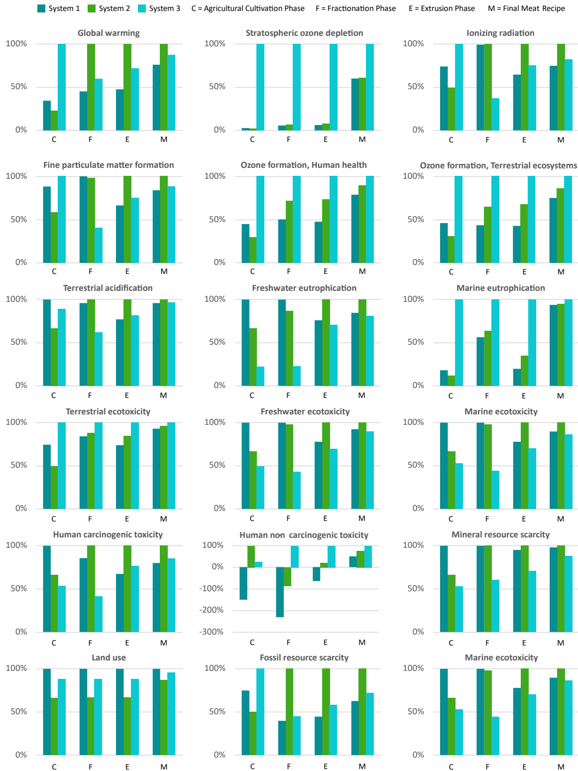
Figure 5-41. Cumulative comparison between Systems #1 to #3, plant-based meat recipes, cradle-to-manufacturing gate. Method: ReCiPe 2016 Midpoint (H) V1.03. Cumulative contribution analysis dashboard per stages for Systems #1–3, plant-based meat systems, cradle-to-manufacturing gate. Method: ReCiPe 2016 Midpoint (H) V1.03. Built based on Figure 5-38 to Figure 5-40.
